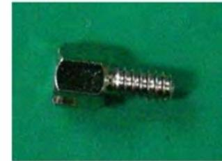
6. Separate 4 6-angle screws under the SHIELD.
