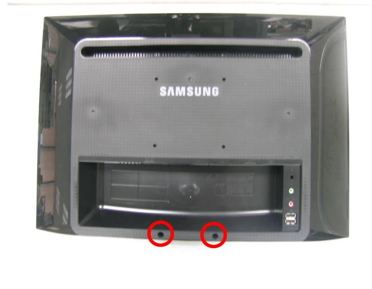
2. Remove the two screws and put hand on stand hall between two screw halls and lift back cover.
