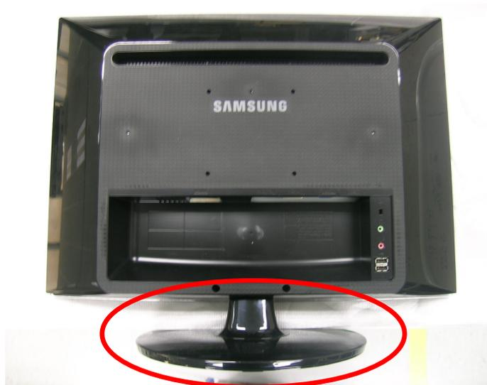
1. Place the monitor on the soft table with the front part facing downwards and remove the stand by pulling downward forcefully.
