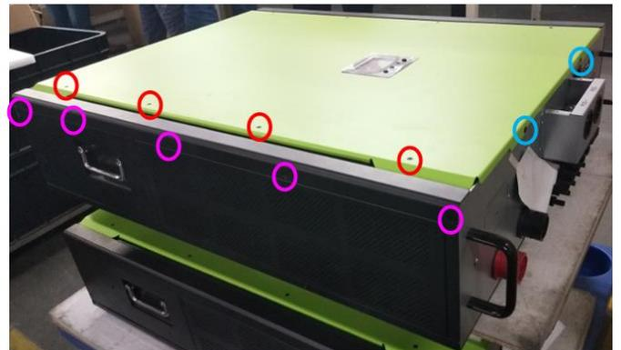
Open the top cover slowly. Before you can open it totally, please don't forget to remove the cables attach the LCD:
